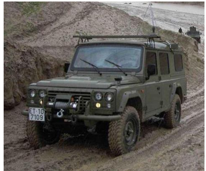
The Santana PS 10 had a 2.8 litre Iveco 8410.43 turbocharged intercooled diesel engine
