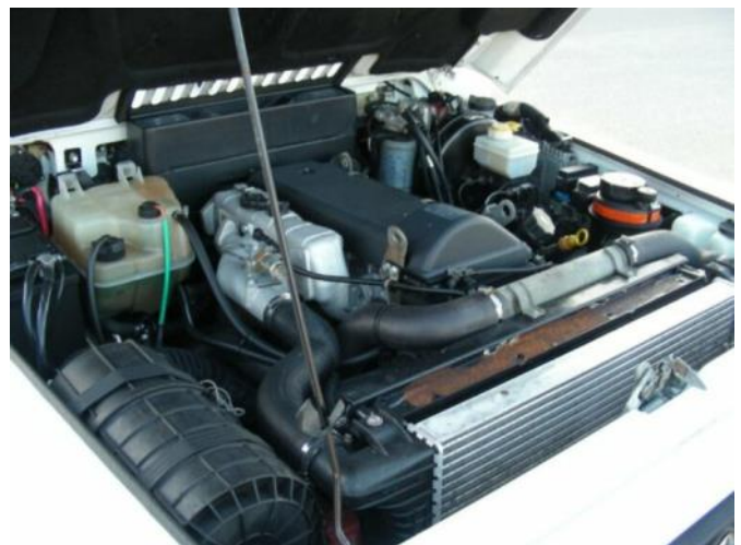
The Santana PS 10 had a 2.8 litre Iveco 8410.43 turbocharged intercooled diesel engine
