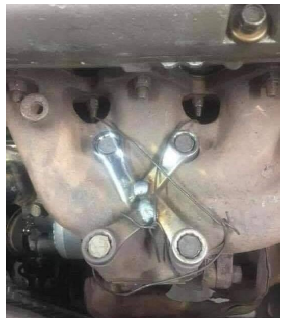
Hoody has worked out how to keep those bolts from coming undone
