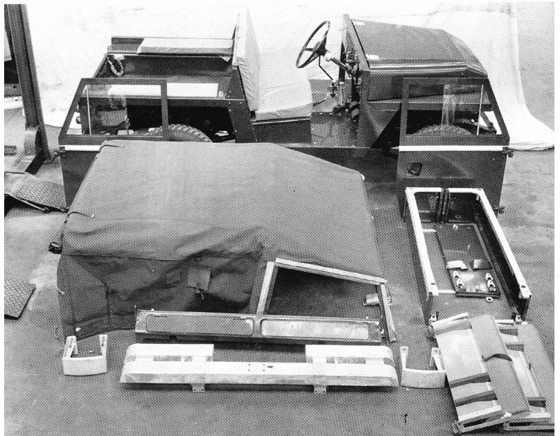
Publicity photo of first prototype showing the parts that could be removed to get the vehicle into the "Lightweight" form.
